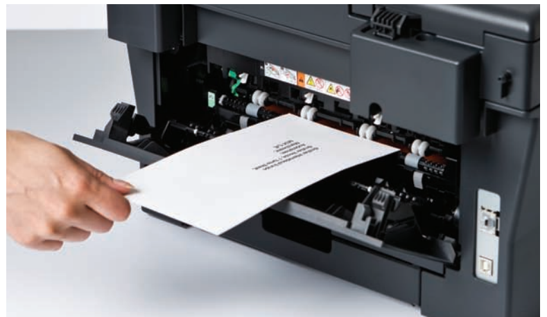
Print on thicker media and envelopes using the manual feed slot
